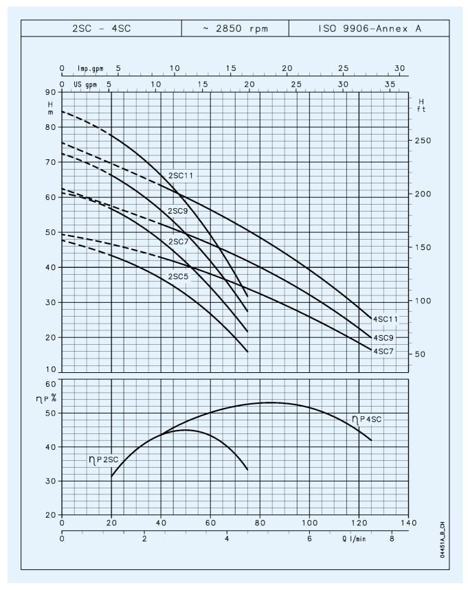
These performances are valid for liquids with density  $\rho=1.0$  kg/dm³ and kinematic viscosity  $\gamma=1$  mm²/sec. \* Named SC for UK market.
