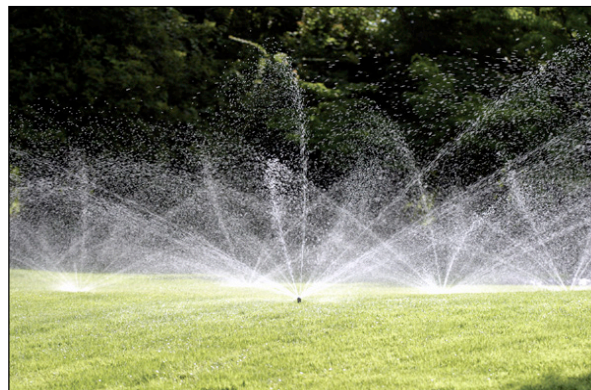
Figure 2. Multi-Stream, Multi-Trajectory Rotating sprinklers distribute water in individual streams, which turn slowly.
