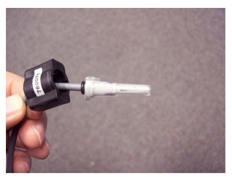
Insert the reed switch into the register:
