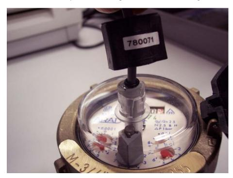
Push down the bayonet and rotate it clockwise to lock the reed switch:
